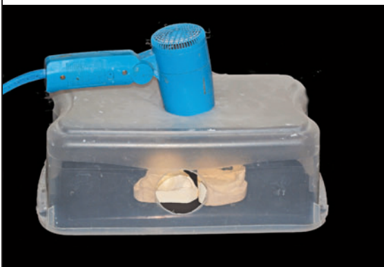
Fig. 5a A drying box constructed from a dollar store box and a hair dryer shortens the drying time of models and the coatings of Wondergloss to 10-15 minutes. Holes cut on sides allow for air flow through and also prevents the dryer's thermal sensor from overheating.
