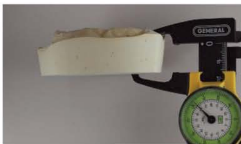
Fig. M The model should be 15-16 mm at its thinnest point.
