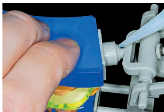
Fig. 11 Glue upper ball joint together
