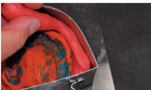
Fig. E Use excess material to backfill.
