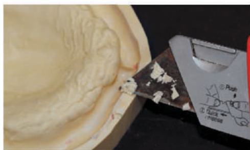
Fig. K Final trimming is accomplished with model trimmer to define model dimensions, and a razor knife to smooth land areas.
